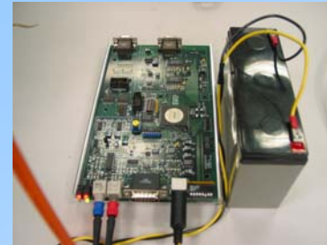
Remote ADC unit and battery
