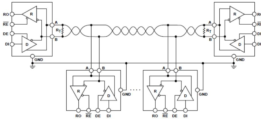
Figure 3. Half-Duplex RS-485 Bus Configuration
