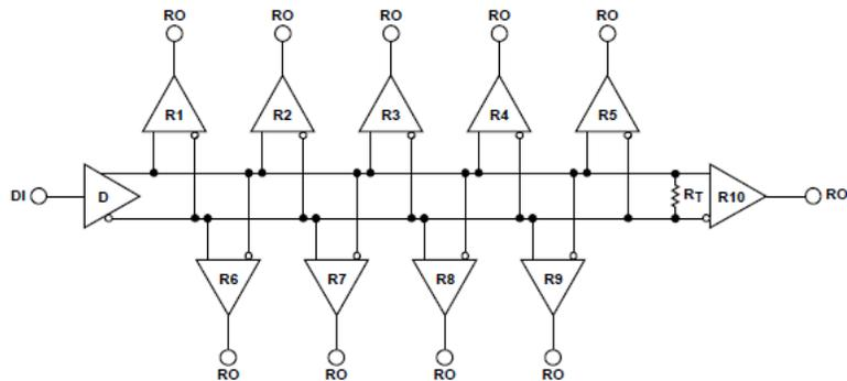
Figure 2. Typical RS-422 Interface Circuit
