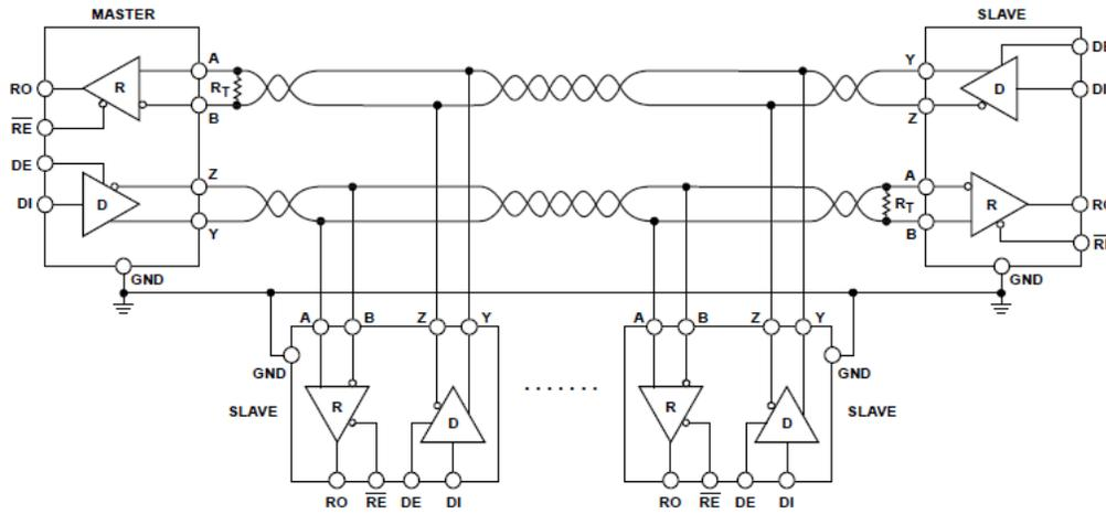
Figure 4. Full Duplex RS-485 Bus Configuration
