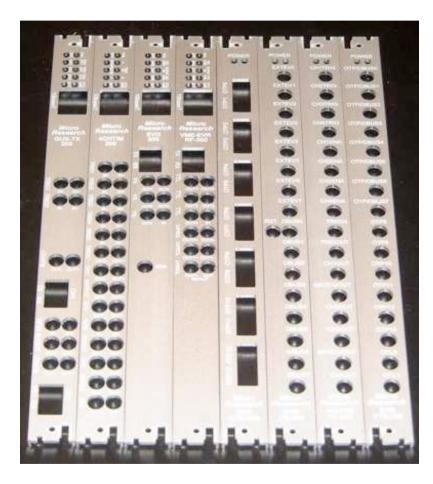
EGUN-Tx (EVR with links to an e-gun trigger card (low jitter, < 1ps) 4-channel precision timer (10 ps resolution) Event Generator EVR with RF recovery
