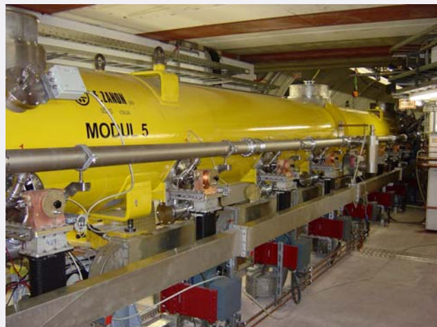
M5 Test with RF, Q_0 = 8 \cdot 10^9 at 25 MV/m
