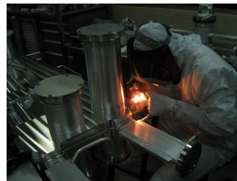
Bending chamber in auto-welding stage
