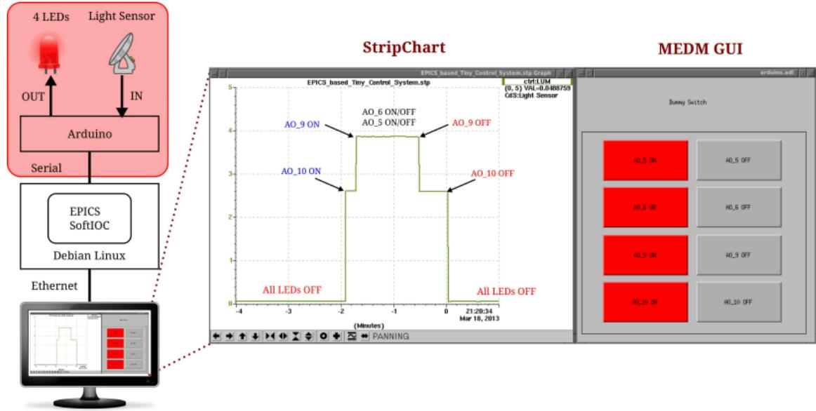
A plan is to build a basic example to learn EPICS by using PC, Arduunio, LED, and one light sensor. (Cheap and Simple)
