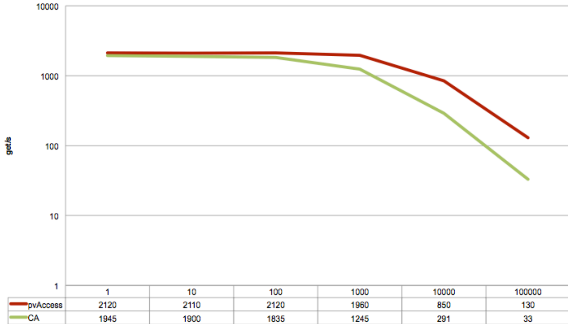
One channel, double array element count on x axis
